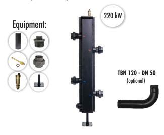
Hydraulic separator CPN 120 is made of steel. The factory is equipped with insulation, and the upper side with two connections for the temperature sensor and a vent (coupler 1/2 " M), and the lower side of the drain connection (coupler 2" M). In the set they are automatic air vent  $\frac{3}{8}$  " with check valve  $\frac{1}{2}$ ", immersion sleeve for temperature sensor 1/2", four cast-iron fittings 2" and mounting feet.
